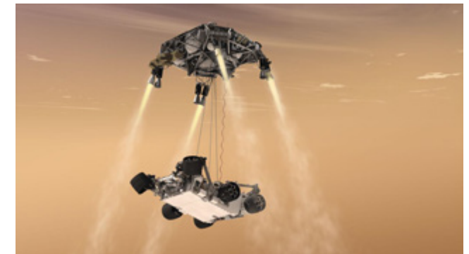
Figure 1. Final stage of landing of the Curiosity launched by Mars Science Laboratory of NASA in 2011
